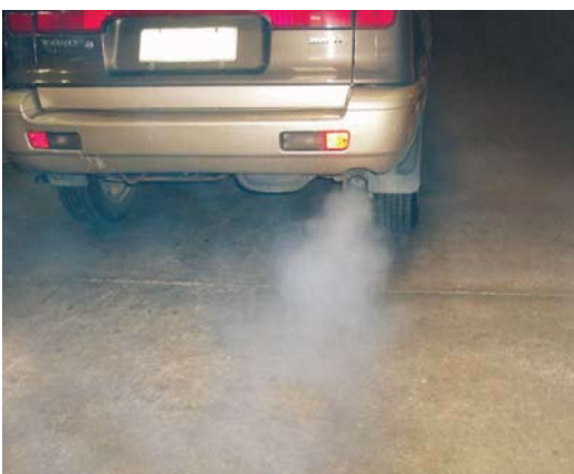
Figure 4. Clearly visible smoke. This vehicle would fail.
