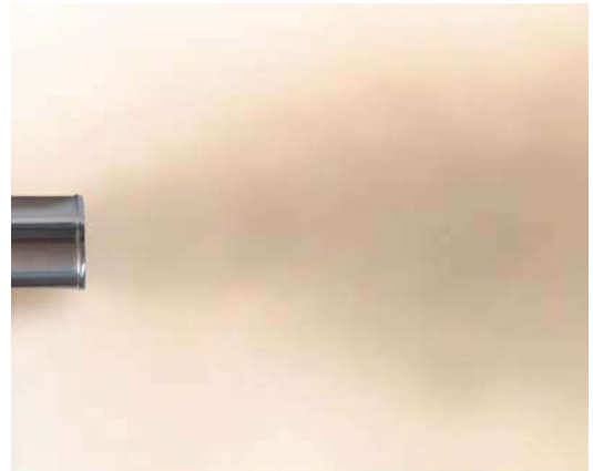
Figure 3. Clearly visible smoke. This vehicle would fail.
