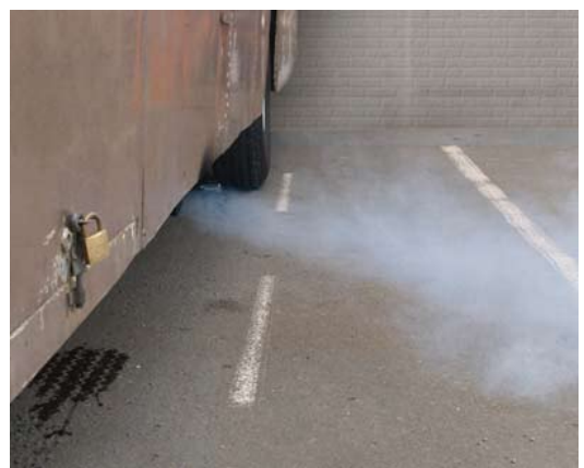
Figure 5. Clearly visible smoke. This vehicle would fail.
