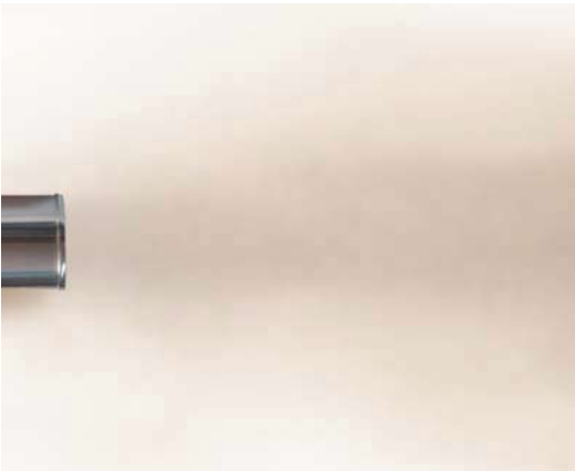
Figure 2. Clearly visible smoke. This vehicle would fail.
