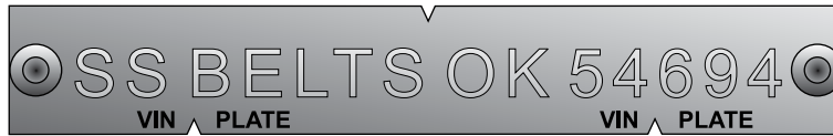
Figure 7-5-6. Example of plate fitted to a vehicle that may retain single-sensitive front seatbelts
