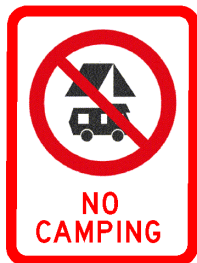
Example R5-8 “No camping” sign
