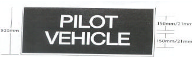
Figure 4 Warning sign for pilot vehicle [Refs. 7.3(9), 7.3(12)]
