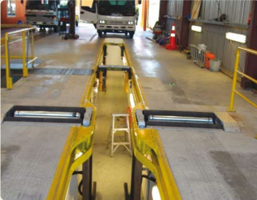
The new Maha roller brake machine with chassis load simulation.
